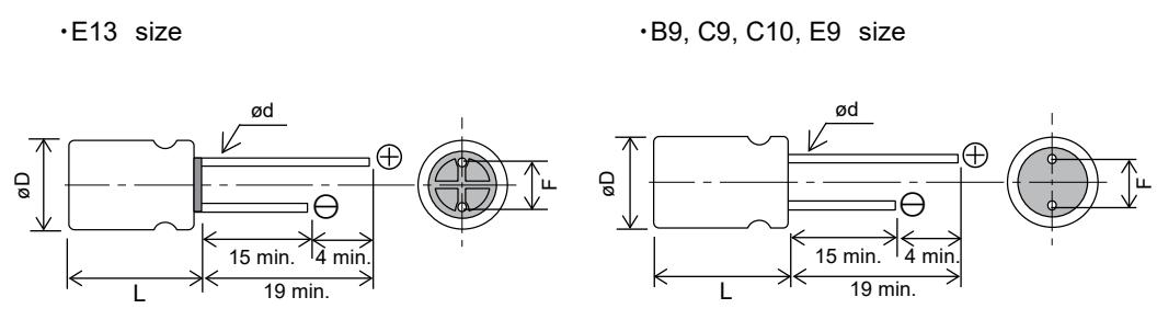
Flat rubber is used for B9, C9, C10, and E9 size.
