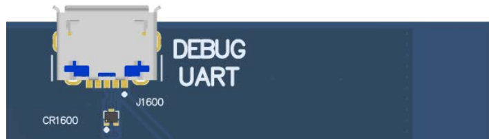
Figure 11. Debug UART over USB J1600
