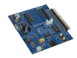
The DIGI XBee® XBIB-C-MMT Development board uses a secondary USB connector and has switch controls whether
